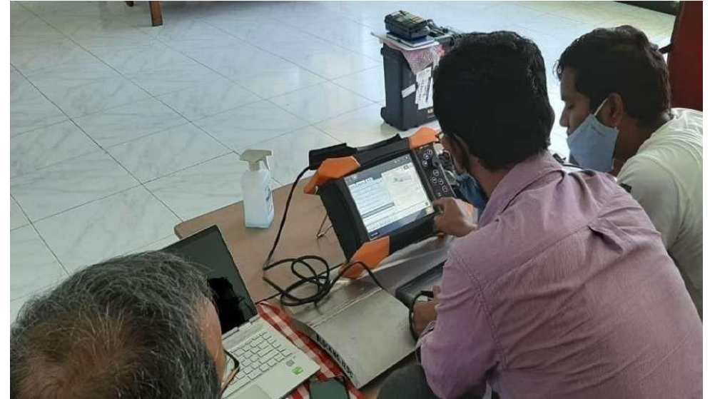
Demonstration of Plain Wave Imaging technique advance PAUT inspection for the detection of IGSCC in stainless welds in the presence of NPCIL team at TAPS 1&2
