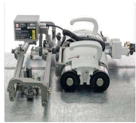
Stegrover Fully automatic scanner with weld tracker
