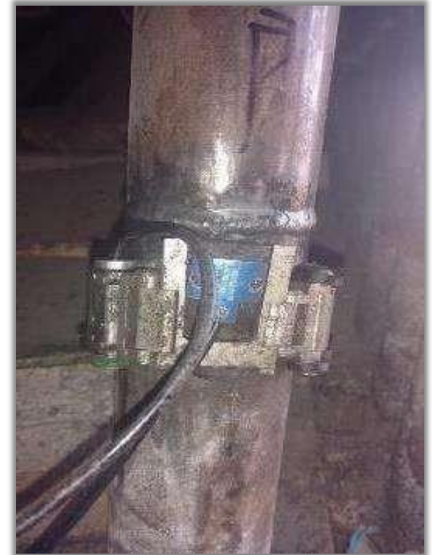
PAUT of Power Plant Piping Using Cobra Scanner at Sonichar, NIGER
