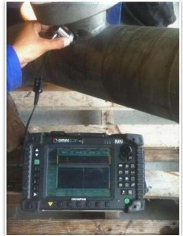
PAUT Inspection of Spool at Aker Solutions, India
