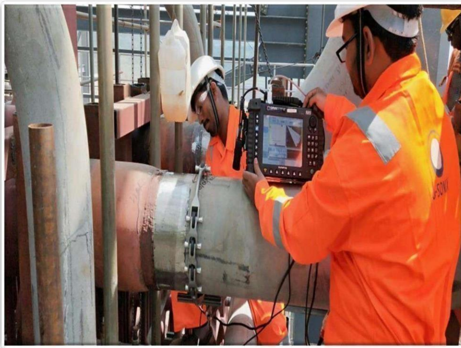
PAUT Inspection of Piping Joints at HQ Peat Power plant, Rwanda, Central Africa
