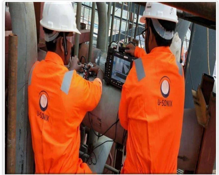
PAUT Inspection of Piping Joints at HQ Peat Power plant, Rwanda, Central Africa
