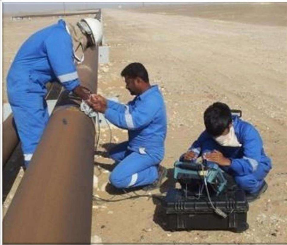
PAUT Inspection Of Pipelines for PDO Oman
