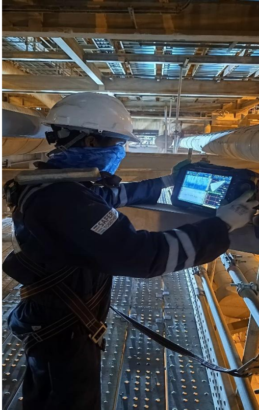
PAUT Inspection of Furnace Pipes and Vessels at Yanbu Aramco Sinopec Refining Company (Yasref) Ltd, Kingdom of Saudi Arabia
