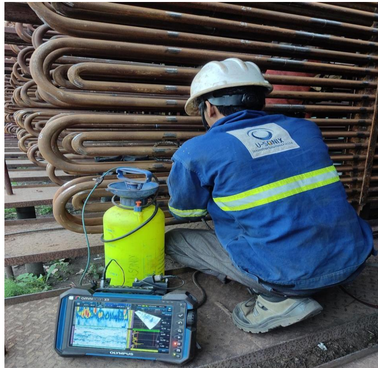
Boiler Tube Inspection at TATA Power, Jamshedpur, India
